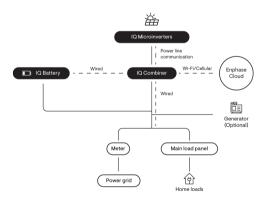
Figure 4: Grid-tied system configuration
