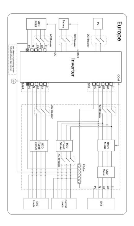
The wiring system of the basic application is an example for grid systems without special requirement:
